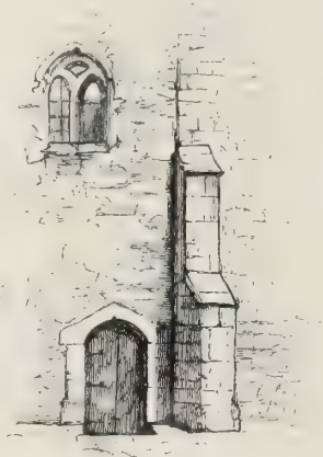
Fig. 7. Buttress at junction of Hall and Kitchen.
